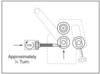
Figure 16. Raising bottom roller <sup>1</sup>/<sub>4</sub> turn.
